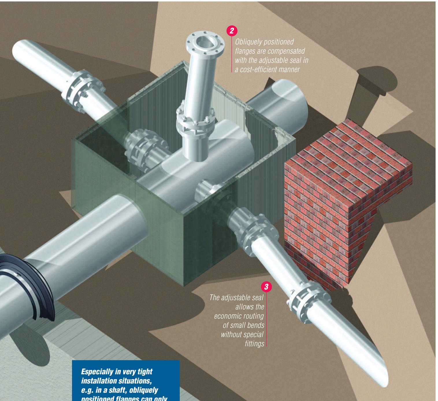
**2** Obliquely positioned flanges are compensated with the adjustable seal in a cost-efficient manner
