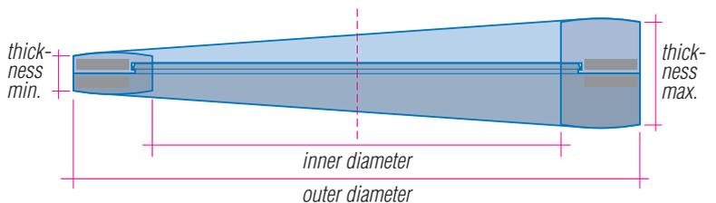
The standard material of the adjustable seal Type KGS/VD is EPDM. However, depending on the applications, it can also be produced of other elastomeres, such as FKM (Viton) or Silicone.
